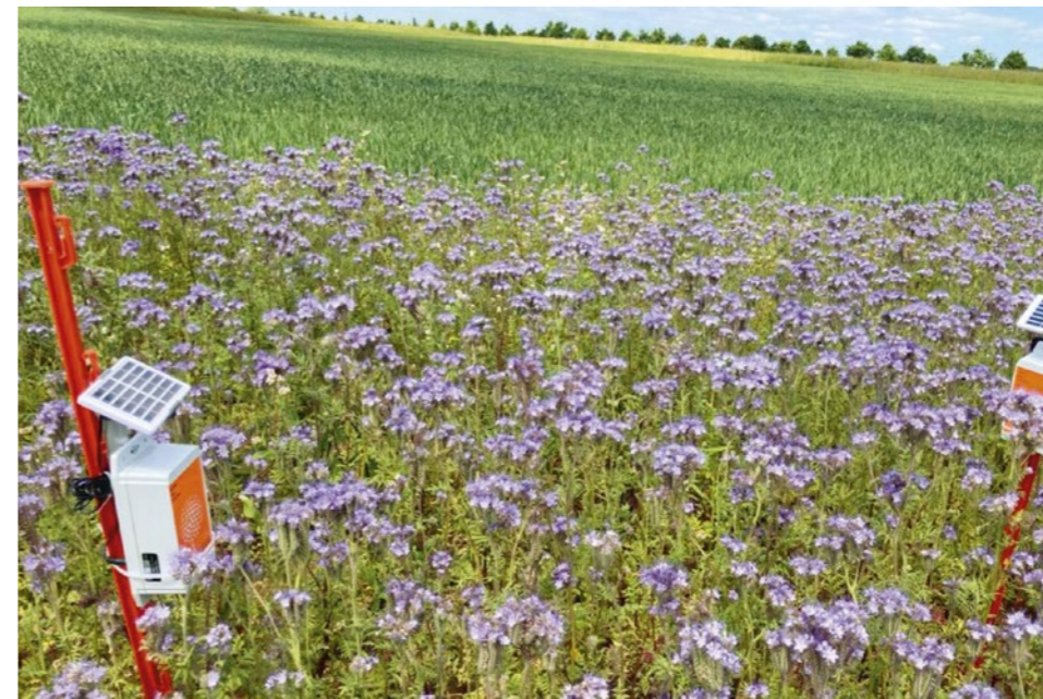
AgriSound detects pollinators, particularly honeybees and bumble bees, using algorithms to translate the wing beat speed and time spent on the plant.
