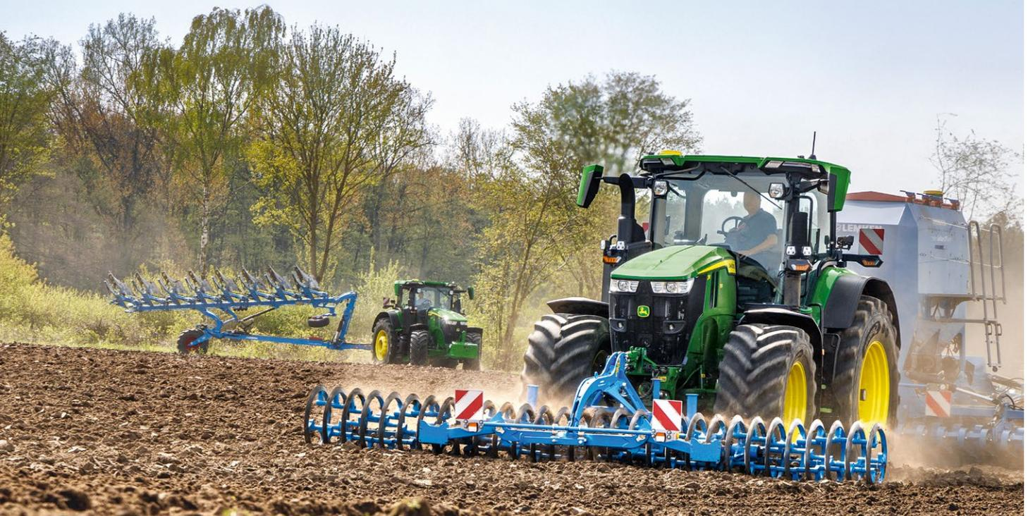
Optionally available, the iTEC™ compatible front hitch has a constant lift capacity of 3,500 kg at the hooks.
