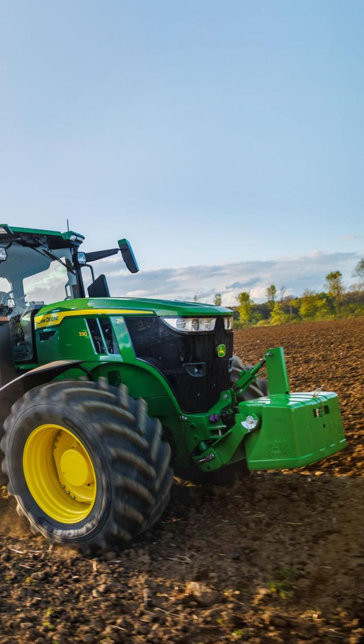
Top field performance – Ten gears in the main working range from 5-16 km/h provide the ideal gear for the most demanding pulling applications.
